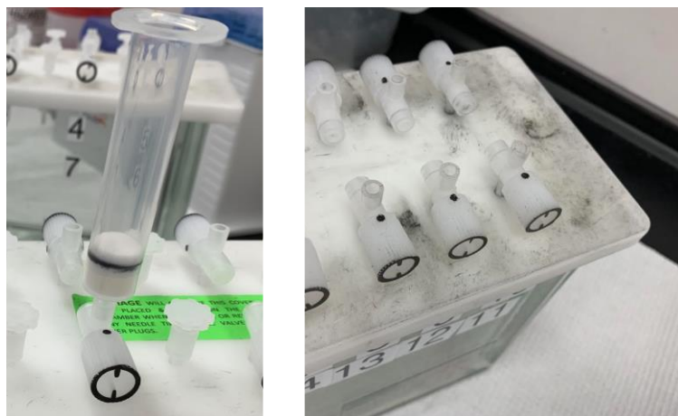
Figure 1. SPE Cartridges Used for the Soil Extract Study versus Loose Carbon.
